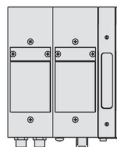
\* The feed-back signal box extends the terminal by 40 mm.
