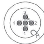
**BUS IN BUS OUT** Socket M12 4-pin D-code
