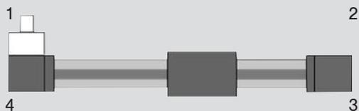
Brake at 1 with extended shaft for synchronization at 1
