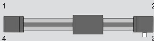
Shaft for encoder connection at 3
