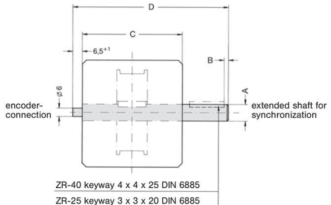
The slide travels 135 mm (Ø 25) per one rotation of the shaft.
