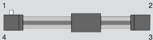
Shaft for encoder connection at 1
