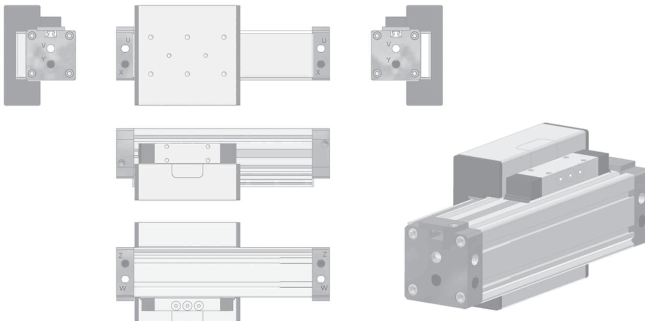
Option -04 enable to connect pressure at both face ends or one face and one side port.
