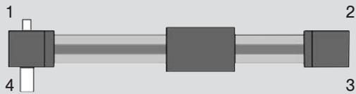
Shaft for encoder connection at 1
