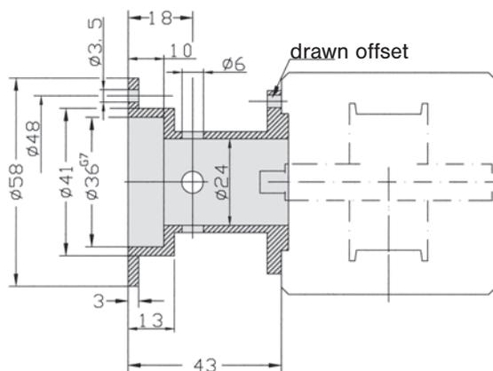
The adapters can be mounted on all cylinders of series ZR and will fit all encoders with a 36 mm centering collar.
