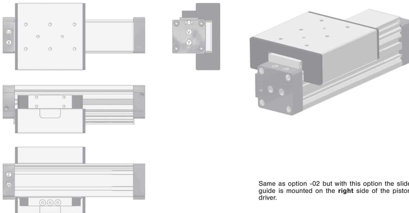
Same as option -02 but with this option the slide guide is mounted on the **right** side of the piston driver.
