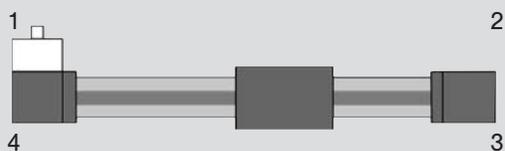
Brake with encoder connection mounted at 1
