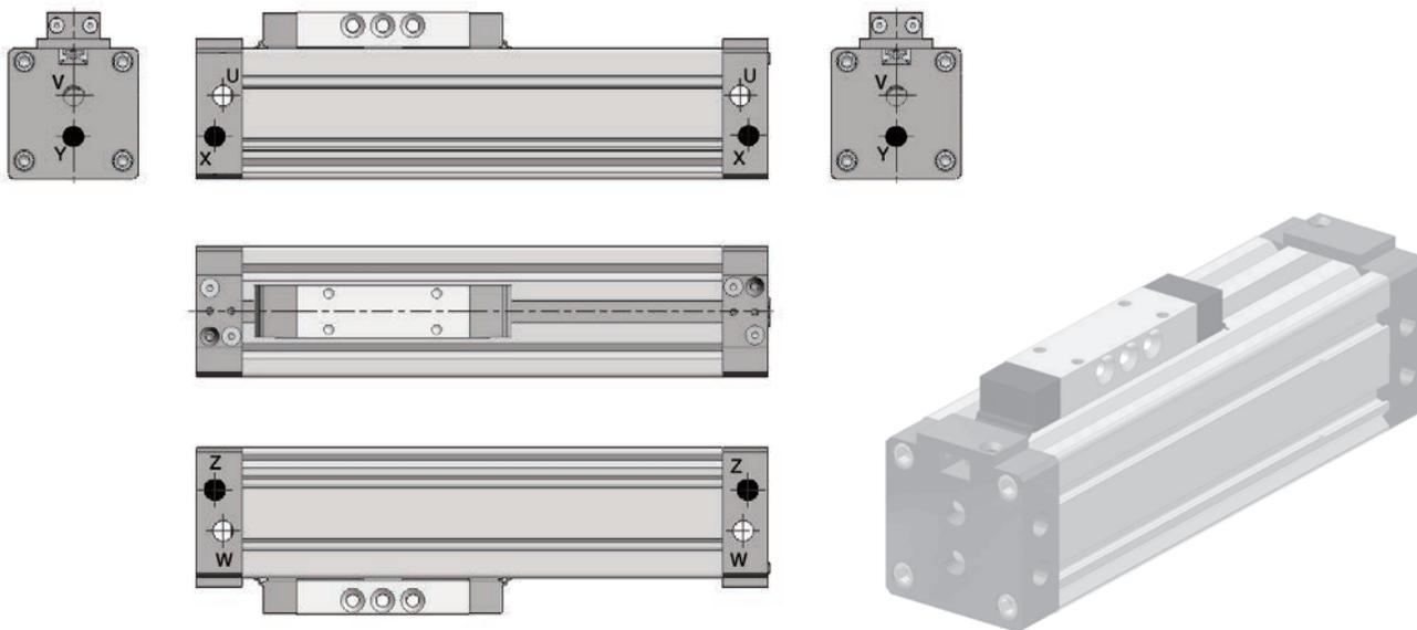
Option -04 enable to connect pressure at both face ends or one face and one side port.
