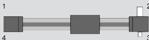
Shaft for encoder connection at 3
