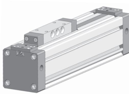
Option -01 cylinder comes with two pressure connections (W-X and Y-Z respectively) on each end. User is required to select one of two pressure connections on each end. Second port will require the installation of a sealing plug (2 plugs are supplied).
