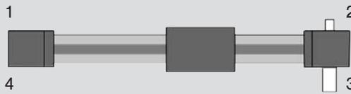
Shaft for encoder connection at 2
