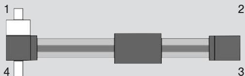
Brake at 1 with shaft for synchronization at 1 and 4
