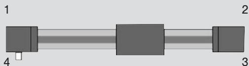
Shaft for encoder connection at 4
