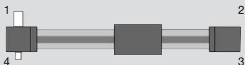
Shaft for encoder connection at 4
