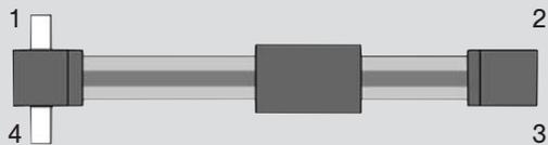
Shaft for synchronization on two sides
