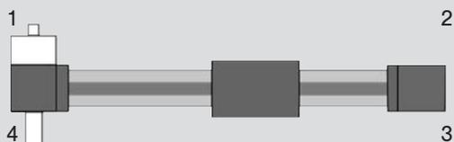
Brake at 1 with extended shaft for synchronization at 4
