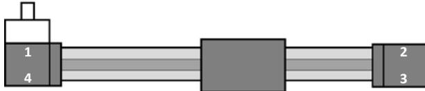
Brake at 1 with extended shaft for synchronisation at 1
