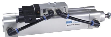
Double acting Al-profile cylinder with integrated sensor grooves, adjustable cushions and magnetic piston for proximity sensors. The sensors can be installed directly into the sensor grooves of the Al-profile. The cylinder includes a 5/2- or 5/3-way valve with a high flow rate and compact dimensions. Standard stroke lengths in table below, additional lengths on request.
