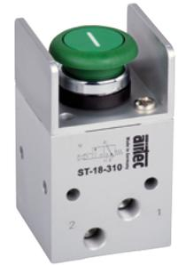
Servo-operated spool valve with low actuating force. The actuating is constantly pilot air supported and is venting\* in resting position on a small amount of air. \*(through a gap between holder and body)
