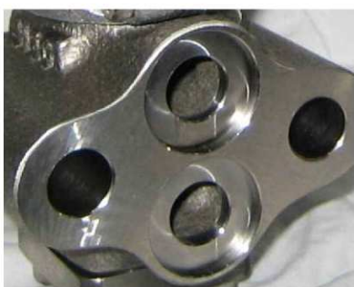
Figure 4. Grooves in Panel Valve for gaskets
