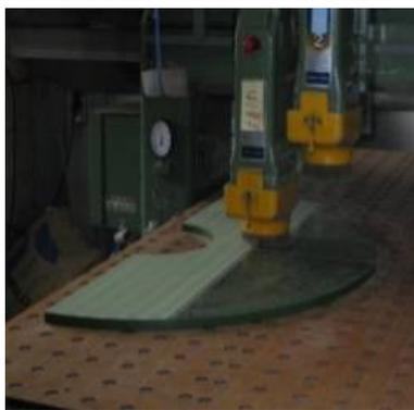
Machining process (No. 1 router) for surface grinding
