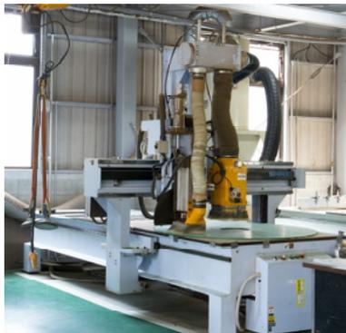
Machining process (No. 2 router) for shape machining
